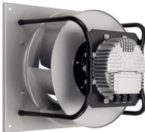
The other important element in an AHU retrofit solution is the replacement of traditional forward / backward curved centrifugal fans with an AC motor with EC fan-motor. EC stands for Electronically Commutated which basically means it is a Fan with a brushless DC motor. Basic DC motors rely on carbon brushes and a commutation ring to switch the current direction, and therefore the magnetic field polarity, in a rotating armature.
